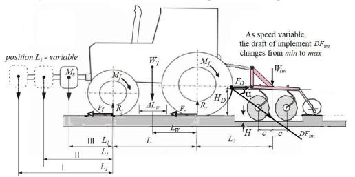
Fig. 3. Scheme of aggregate and acting forces,  $L_2 = 1.8 \text{ m}$ ,  $M_B = 120 \text{ kg}$
